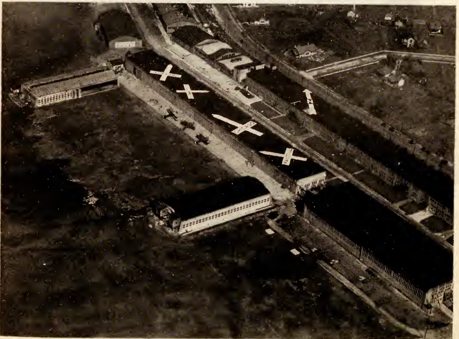
The Air Traveller has no trouble in getting his bearings while flying over Dayton, Ohio. On the hangars at McCook Field are painted great white pointers marking the compass courses to all of the principal cities on the airways in a radius of 500 miles..
